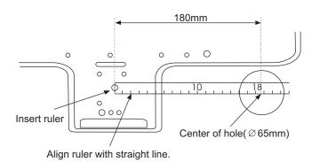
• Confirm the position of holes, and drill holes of  $\emptyset$  65mm on the wall.
