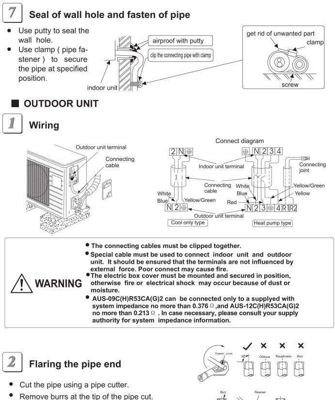
Insert a flare nut into the pipe and modify flare.
